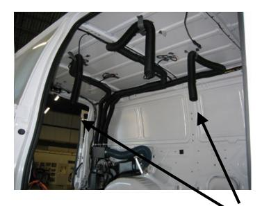
Attach the "Y" duct hose adaptor to the 8 foot front duct hose and connect both 4 foot hoses from "Y" to vents in driver and passenger side front ceiling. This will provide a total of four ceiling vents.
